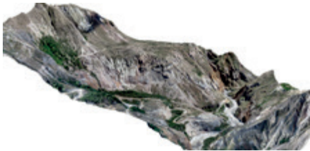
The team's full orthomosaic, overlaid on its 3D DTM of the site
